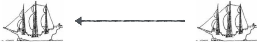
**Egomotion estimation:** the process of estimating the motion of a rigid body using measurements from sensors attached to the body
