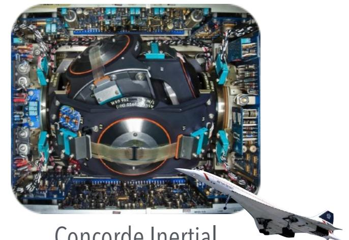
Concorde Inertial Measurement Unit
